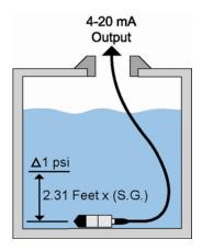
For liquids with a different SG, simply divide 2.31 by the new SG to determine the new ratio. For example, the LD31-S001 is installed in a liquid with a SG = 0.85. The new ratio is as follows:
