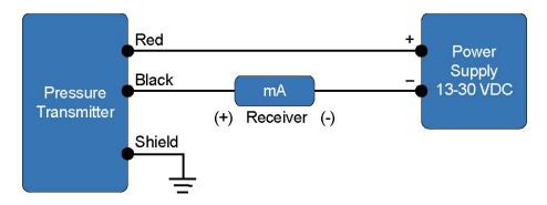
The maximum receiver load resistance (RLmax) for the DC power supply voltage (Vsup) is expressed by the formula:
